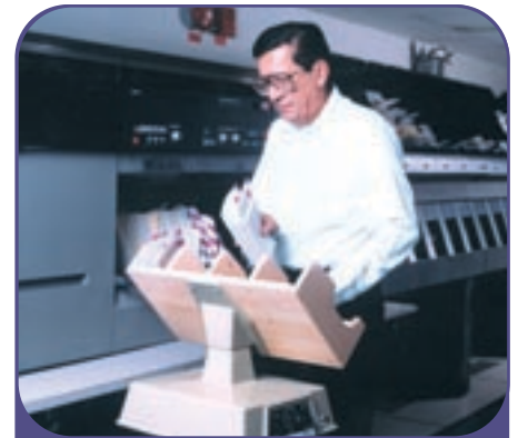
Syntron J-50 4-pocket, shown here, aligning checks prior to insertion into the Lundy Machine.
